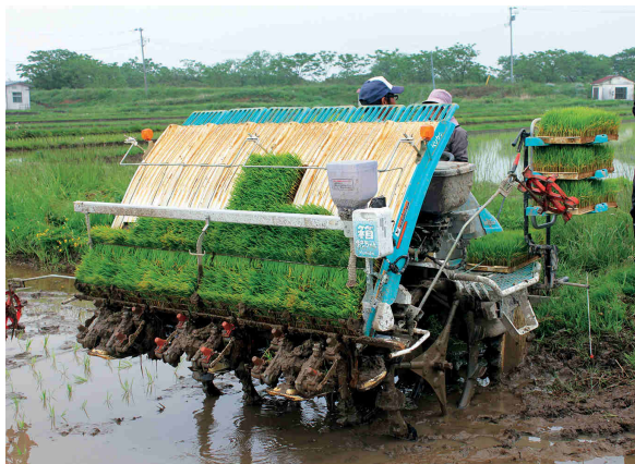
Figure 3. Rice transplantation from nursery boxes into the paddy field. The small white box at right contains insecticide which is dusted on rice seedlings at the time of planting.
